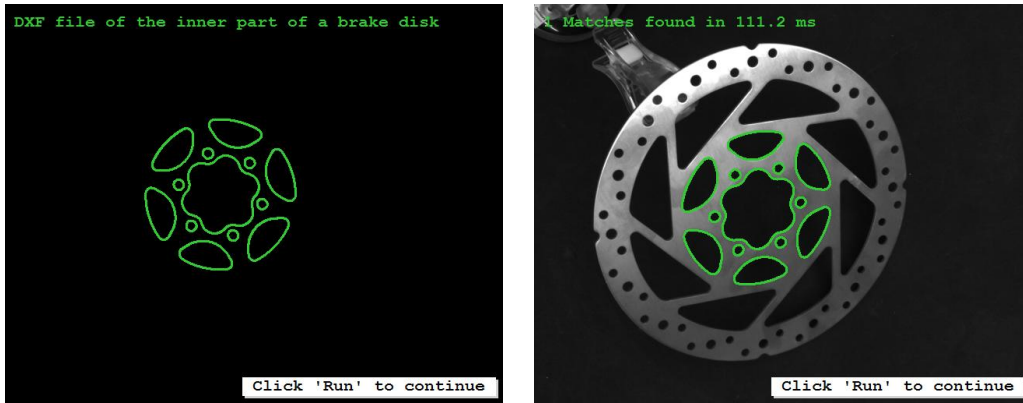
Figure 2.9: (left) synthetic XLD model accessed from a DXF model; (right) model found in a search image.
