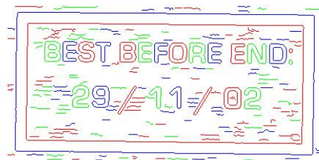
Figure 3.20: Segmentation of initial components with a too low contrast.
