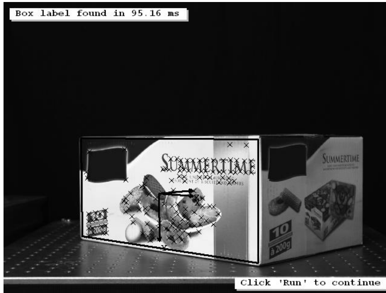
Figure 3.42: 3D pose of cookie box label obtained by calibrated descriptor-based matching.
