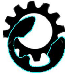
Figure 1.8: Occlusions can be handled by shape-based matching.
