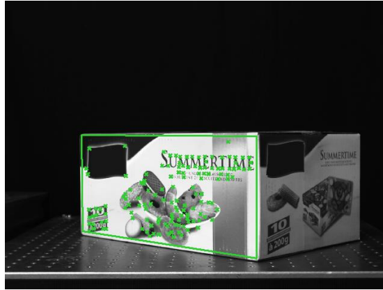
Figure 1.5: 3D object: a plane object part is characterized by a specific texture.
