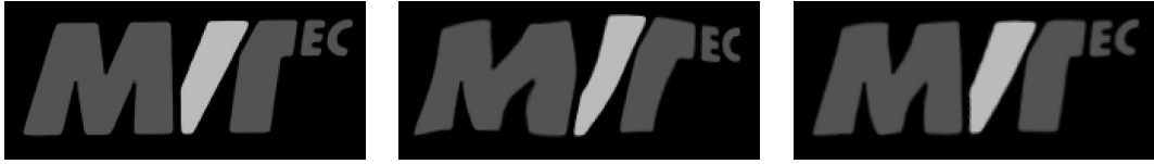
Figure 3.33: From left to right: template image, correspondig part of the search image, rectified image.
