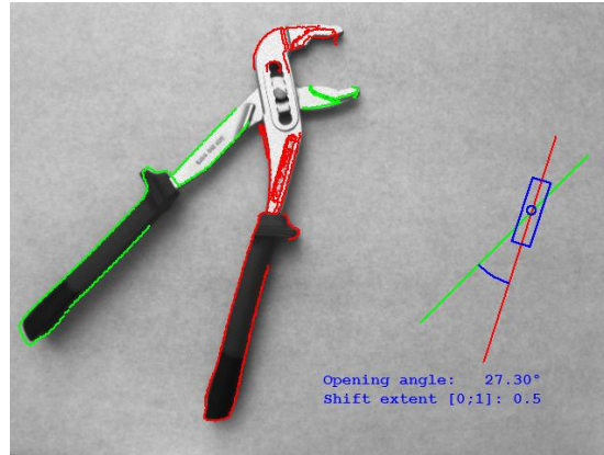
Figure 1.6: Object consisting of two components that move relative to each other.
