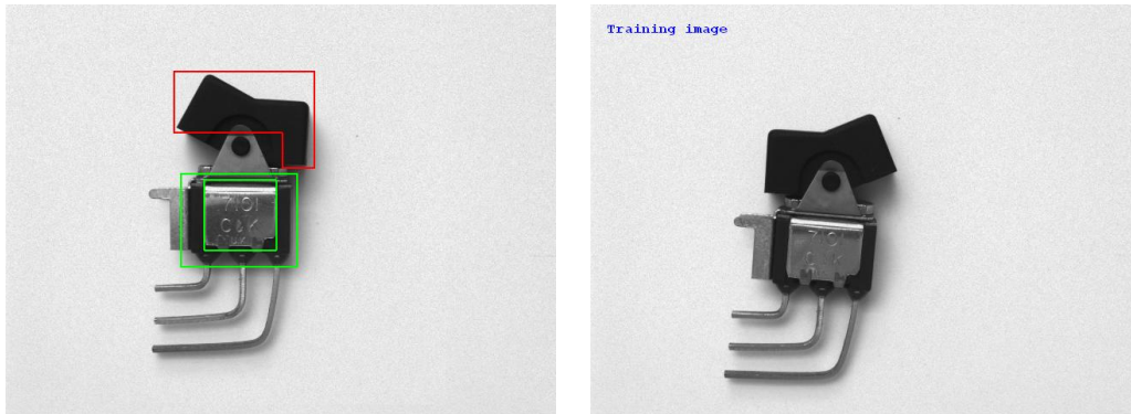
Figure 3.17: (left) reference image with the two initial components (switch is 'on'); (right) training image (switch is 'off').
