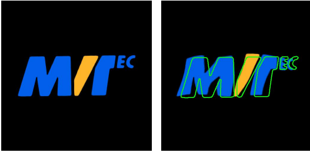
Figure 3.32: (left) “MVTec” logo used for the model creation; (right) deformed logo instance overlaid by the model contours.
