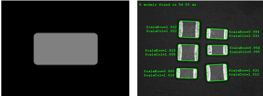
Figure 2.24: (left) synthetic template image; (right) result of anisotropic shape-based matching including the scaling factors in row and column direction.
