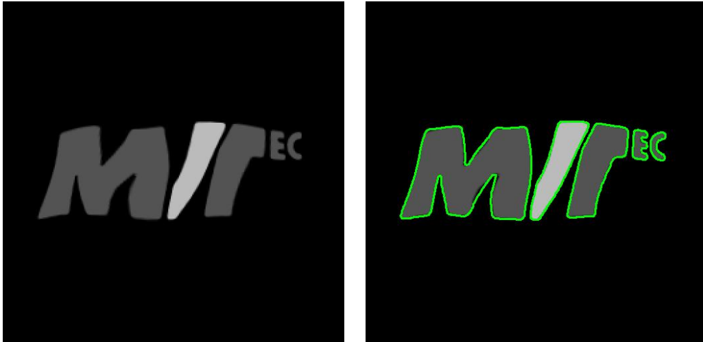
Figure 3.37: (left) search image; (right) search image overlaid by deformed contours.
