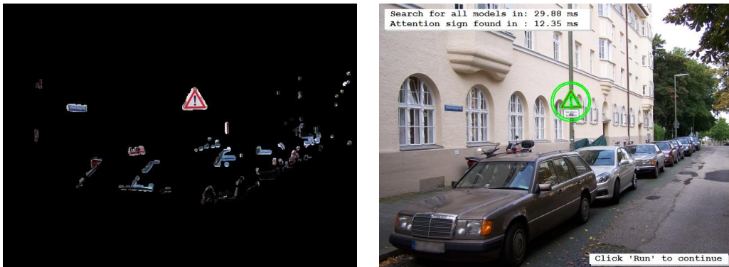
Figure 3.39: (left) ROI derived from the color image; (right) found match for the model of the attention sign.
